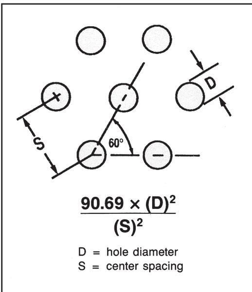
*Fig. 4: Determining the open area in a 45-degree pattern*
