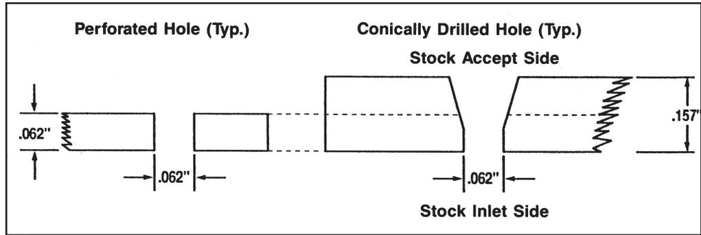
support can be removed. This allows more available screening area. Since the hole is conical in form, fibers pass through in a similar fashion to the perforated hole (Fig. 7).
