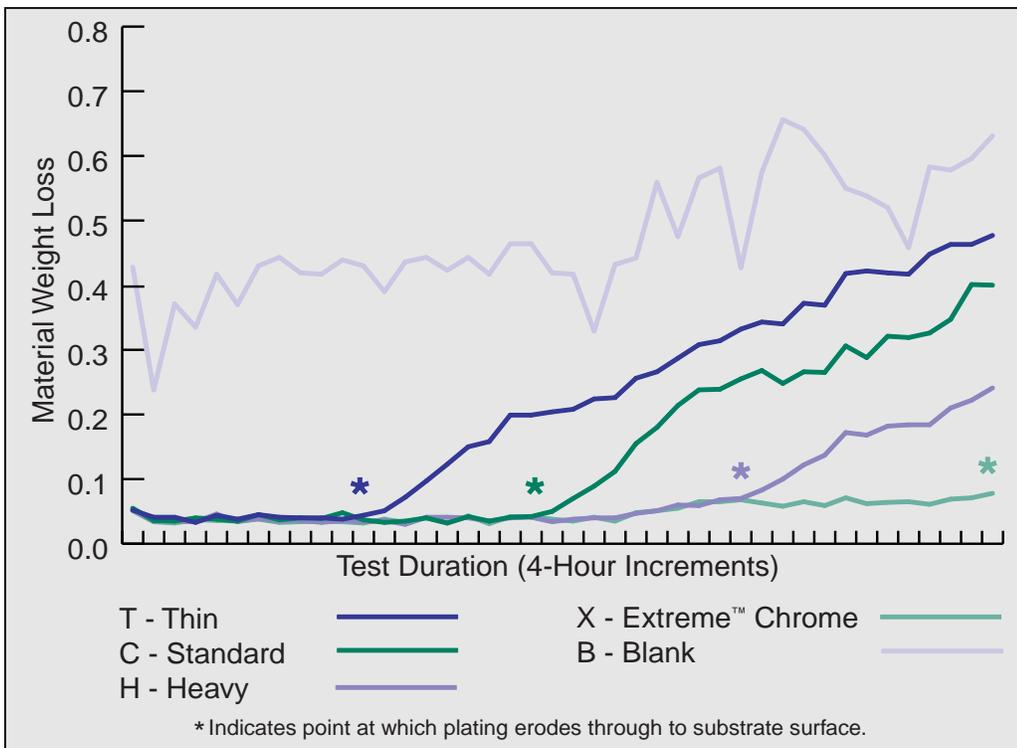
Five samples of 316 stainless steel were subjected to a 168-hour wear abrasion test. Four of the five samples were hard chrome plated at different thicknesses. The fifth sample was not chrome plated and used as a control to measure the effect of the abrasives on standard material. Material loss for each of the samples was measured every four hours. The graph indicates the amount of weight lost in each of the 42 four-hour segments of the trial.
